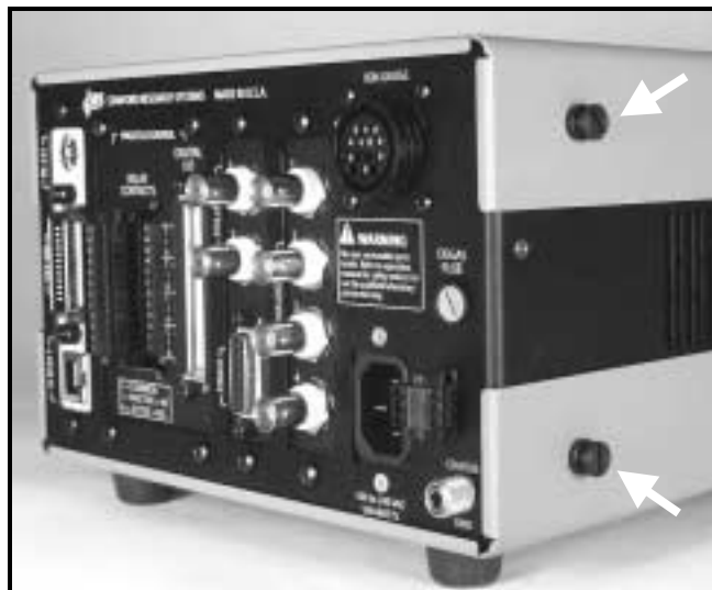
Figure L-3. Mounting pins in place.
